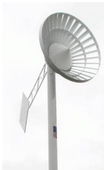
Figure 2.4. The 20-kW EcoWhisper machine (Source: http://www.ecowhisper.com.au/main/page_home.html )
