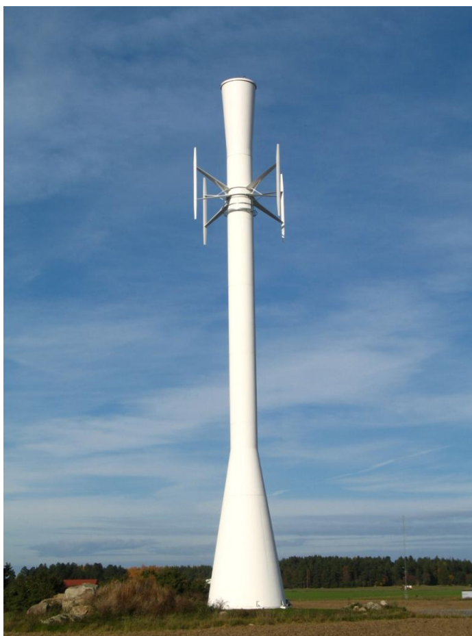
Figure 5.2 Test of a 10-kW VAWT, developed by Vertical Wind in cooperation with Uppsala University for Ericsson. The wind turbine is mounted on an Ericsson Tower Tube, an innovative design that houses base stations and antennas. (Photo: Mikael Bergkvist)
