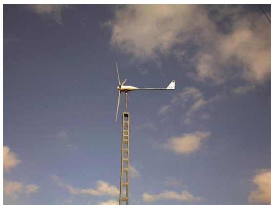
Figure 4.2. Bornay wind turbine Inclín 6 kW
