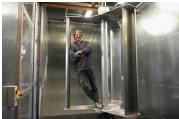
Figure 2.5. Wind tunnel testing of a 20-kW Altaus prototype (Source: http://www.bendigoadvertiser.com.au/news/local/news/general/backyard-generation-gets-grant/1596537.aspx , main Web site: http://www.altaus.com.au/ )
