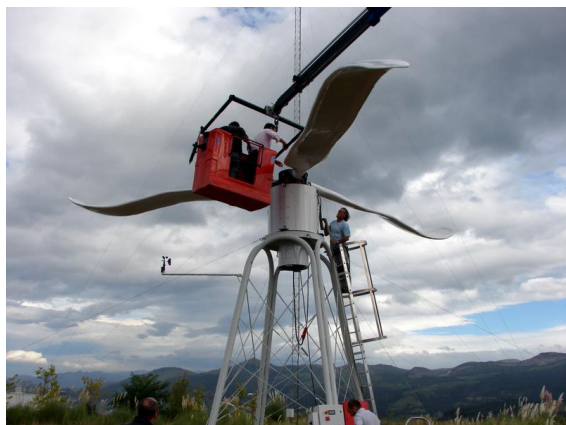
Figure 4.7. 5-kW VAWT prototype developed by INDES MEDIA EOL (PSE-MINIEÖLICA)
